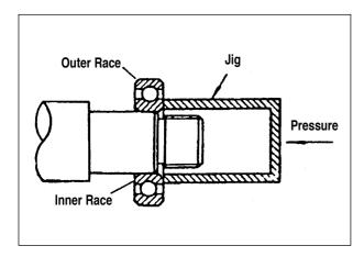
c. When installing a non-split type bearing with necesary interferences of the inner and outer races, use a suitable jig as shown in the figure below to apply the necessary pressure to both the inner and outer races.
